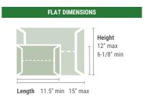
MeasurementMinimum\*MaximumLength11.5 inches15 inchesHeight6.125 inches12 inchesThickness0.25 inch0.75 inch
